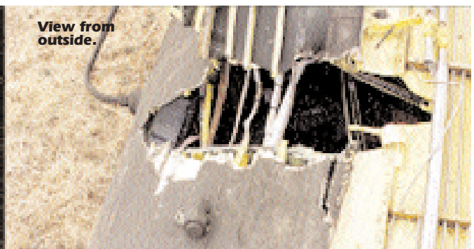
Aft rotor blades tore hole in top of fuselage during emergency shutdown.
