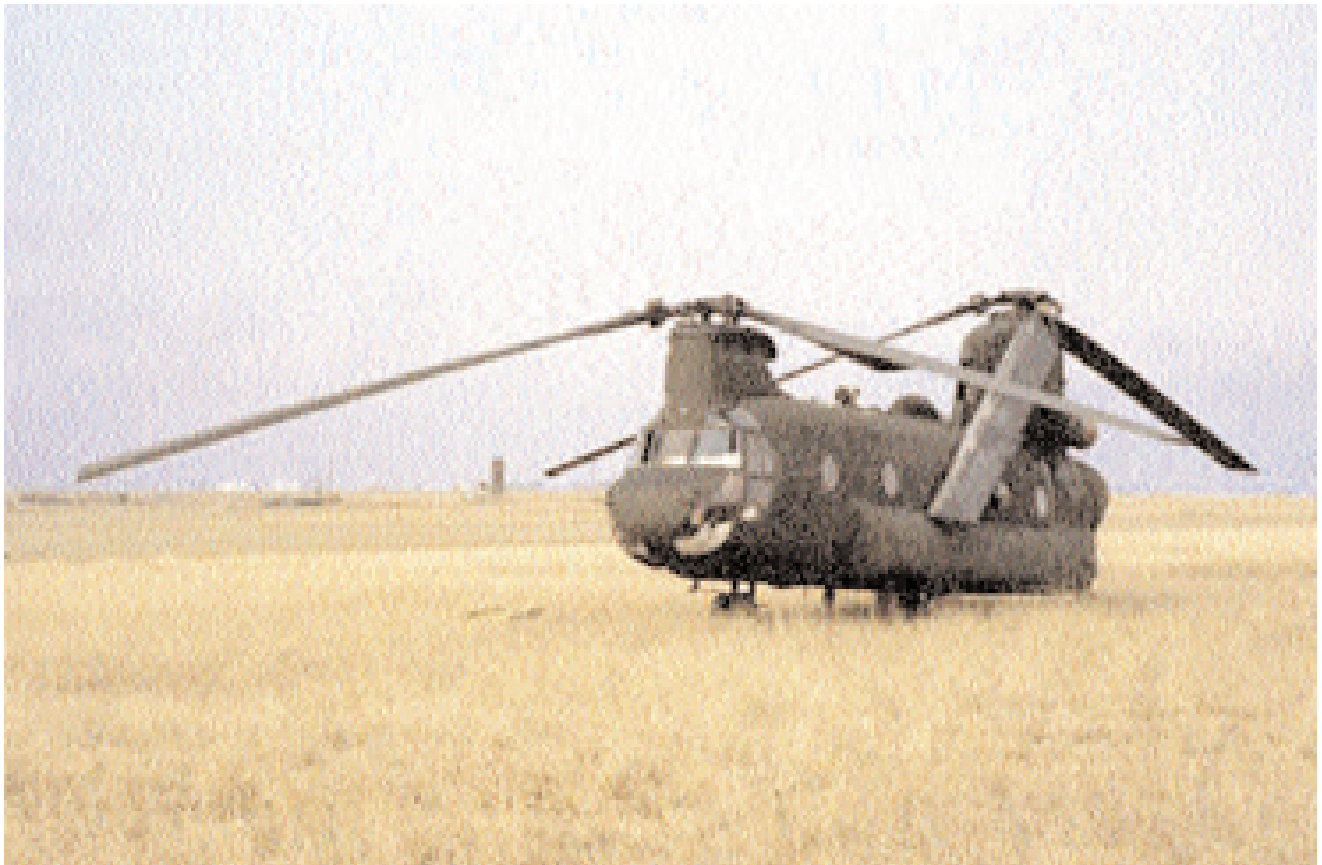
After 360-degree roll in flight, the crew managed to land the Chinook with surprisingly little damage. During shutdown, however, damaged droop stops allowed the aft rotor blades to pound into the fuselage.
